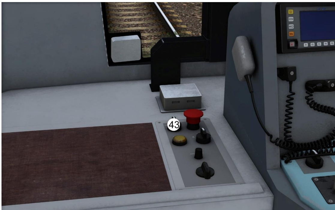
43 Wheelchair lift switch (left, 0, right)
